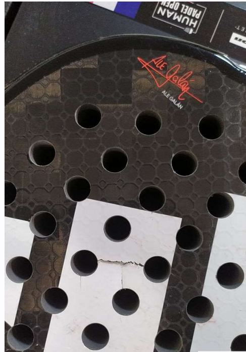
BREAKAGE WITH SUNKEN RUBBER
